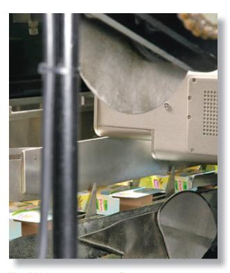
The 7011 laser coders scribe the use-by date and the manufacturing code on 80 to 100 products per minute, depending on the line.
